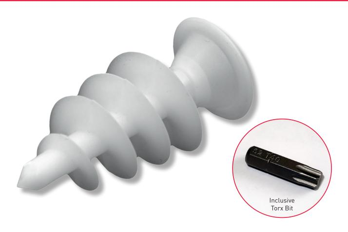
PM MOUNTING SCREW is used to fasten dimpled and drainage membranes to perimeter insulation made of pressure-resistant XPS insulation material. The plastic dowel has a coarse, conical thread and a TX 40 flat head drive
