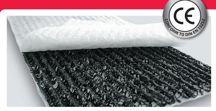
PM 3D-GEOTEX W8 is a strong 8 mm high three-dimensional composite with an exceptionally high drainage capacity. The core consists of robust polypropylene monofilaments with a high void ratio and is combined with a nonwoven geotextile filter on both sides.
